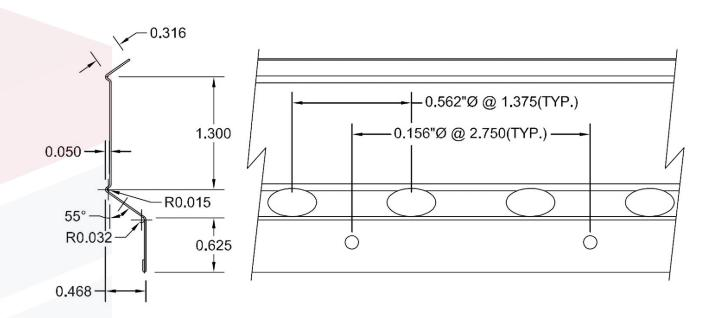
Our metallic resilient bars conform to Canadian steel standards. They are available in standard 12 foot lengths. They are an economical means of reducing noise transmission for wood or metal structural or load bearing partitions.
