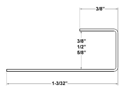
Our metal J trims conform to Canadian steel standards. They are available in standard 10' lengths in 3/8, 1/2"and 5/8" thickness. J trims serve to protect sides of gypsum panels around doors and windows or when gypsum panels rest on other materials.
