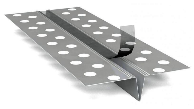
**USE:** To relieve the stresses from expansion and contraction across the joint in large ceiling and wall areas in drywall and veneer finish systems. It is used from floor to ceiling in long partition runs and from door header to ceiling. It is also recommended for repair of existing plastered masonry. Made of roll-formed zinc to resist corrosion, it has 3/32" grounds. Plastic tape protects 1/4" wide x 7/16" deep opening, and is to be removed after installation.
